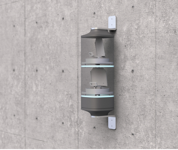
Fig. 2. Small cell with computation core and two beam steering elements
