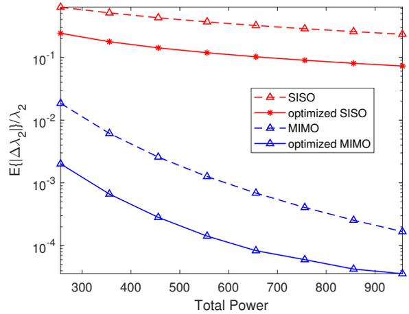
**Fig. 2:** Comparisons between SISO (red curves) and MIMO ( $n = 4$ ) systems (blue curves), with and without optimization.
